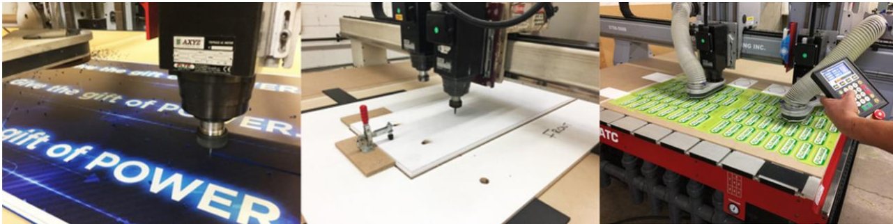
5 CNC tables and a laser that precisely machine many parts at high speed simultaneously
