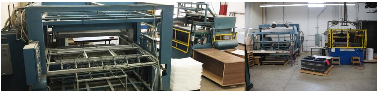
Five large bed vacuum formers, tooling and 100 tonne die punchers that punch perfect shapes with clean edges
